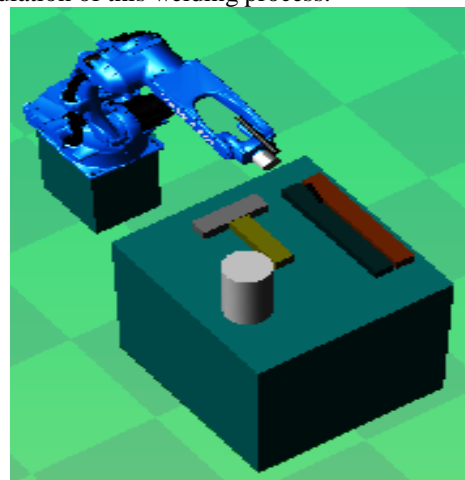
Fig 2. Design of the weld pieces
