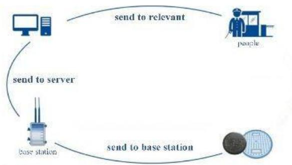
Sewer gas toxicity level detecting sensors, senses the minimum threshold value and ventilates automatically.
