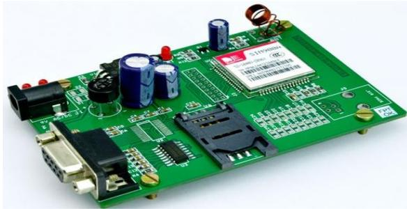
Fig 2: GSM Modem
