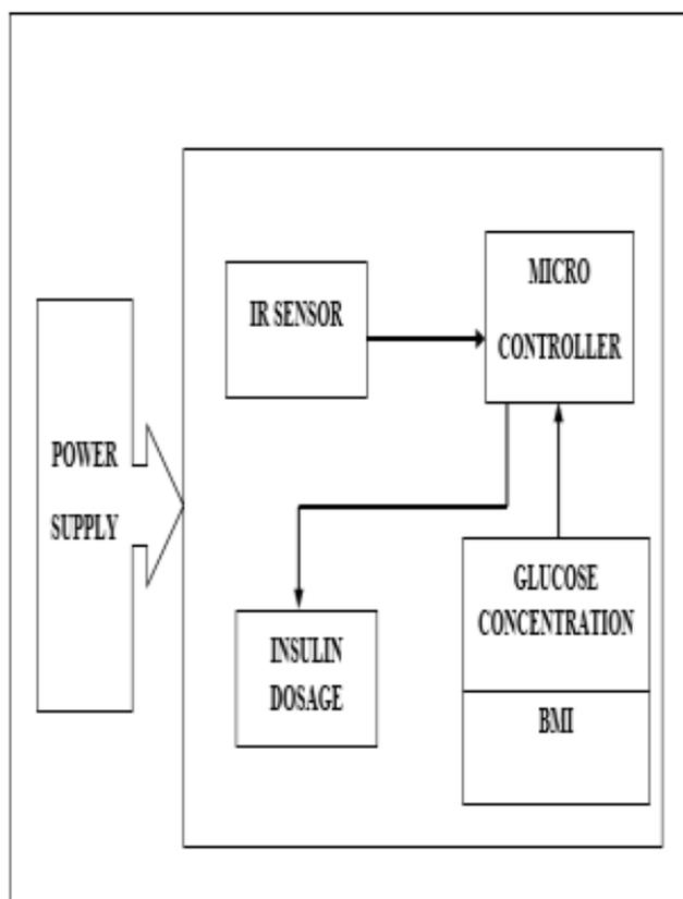
Fig 2: Block Diagram of Automatic Insulin Dosage System
