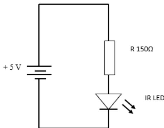
Fig 4: IR Detection (transmitter circuit)
