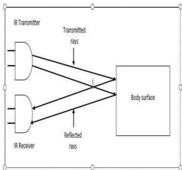
Fig 3: Emission and Reflection of IR LED
