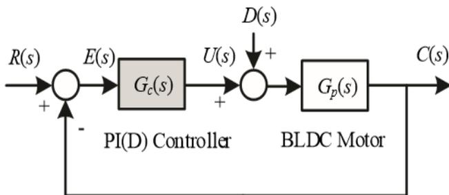
Fig 4 : PI(D) control loop
