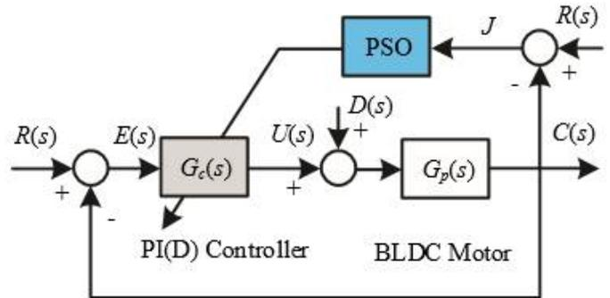
Fig 5 : PSO based PI(D) controller design
