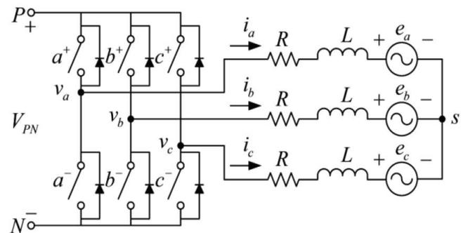
Fig 2 : Equivalent circuit of BLDC Motor
