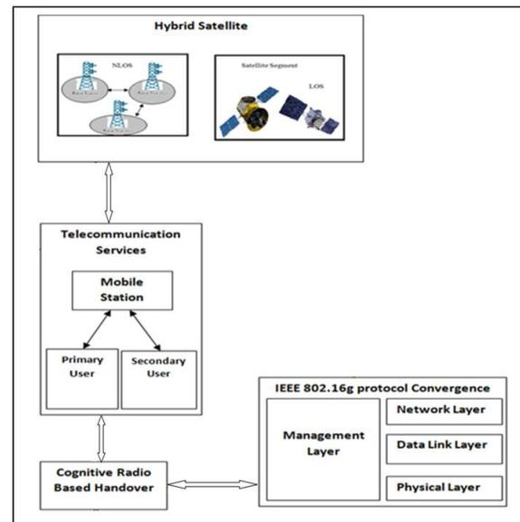
Fig 7: System Architecture of Hybrid Terrestrial Networks
