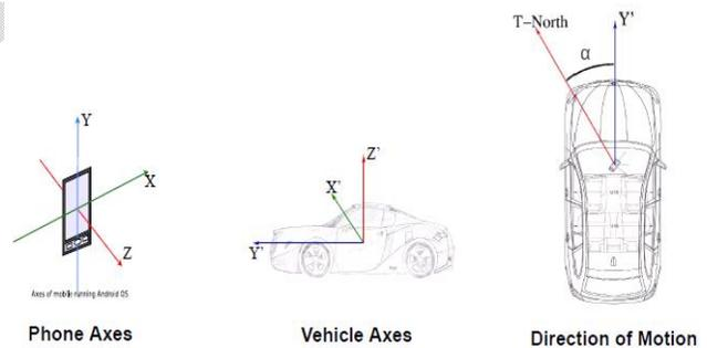
Fig 3 : Representation of co-ordinate Axes.
