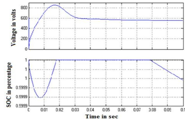
Fig. 5 : Battery Voltage and State of Charge
