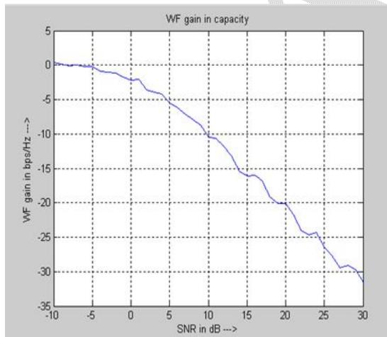
Fig 7 : Water filling gain (vs) SNR
